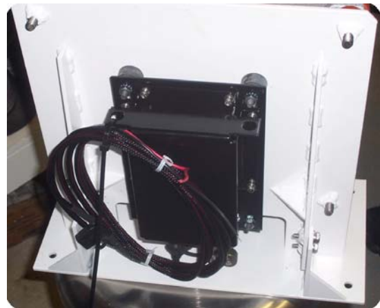
Figure 6. Haul truck mounting plate with BreadCrumb
