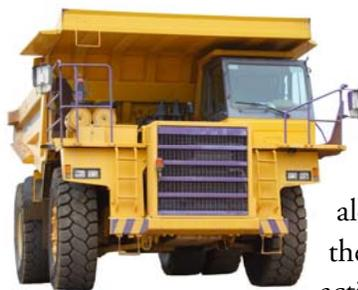
If VIMS detects an impeding or abnormal condition in any of the machine's systems, it will alert the operator and instruct them to take appropriate action, whether it is to modify machine operation, notify the shop of needed maintenance, or perform a safe shutdown of the machine. This improves availability, component life and production while reducing both repair cost and the risk of a catastrophic failure.
