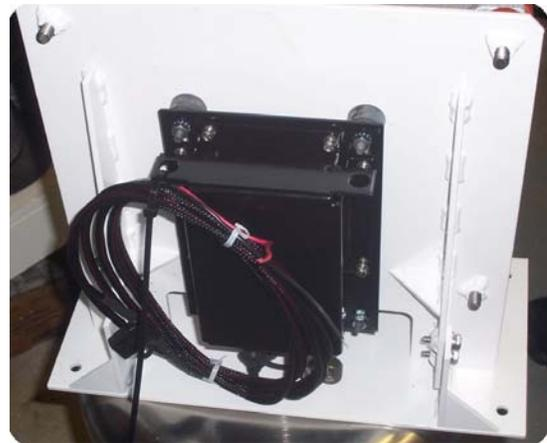
*Figure 6. Haul truck mounting plate with BreadCrumb*
