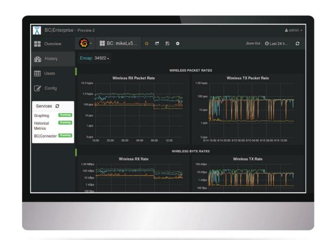
BreadCrumb dashboard screen displaying received and transmitted packet rates over designated time period.
